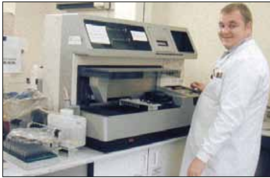
Biochemist in the process of analysing albumin in urine using an autoanalyser.
