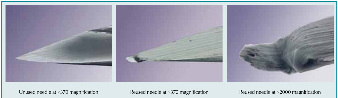
Figure 2. Photographs showing the type of damage that can occur to a needle with reuse. (Source: Look and Strauss, 1998)
