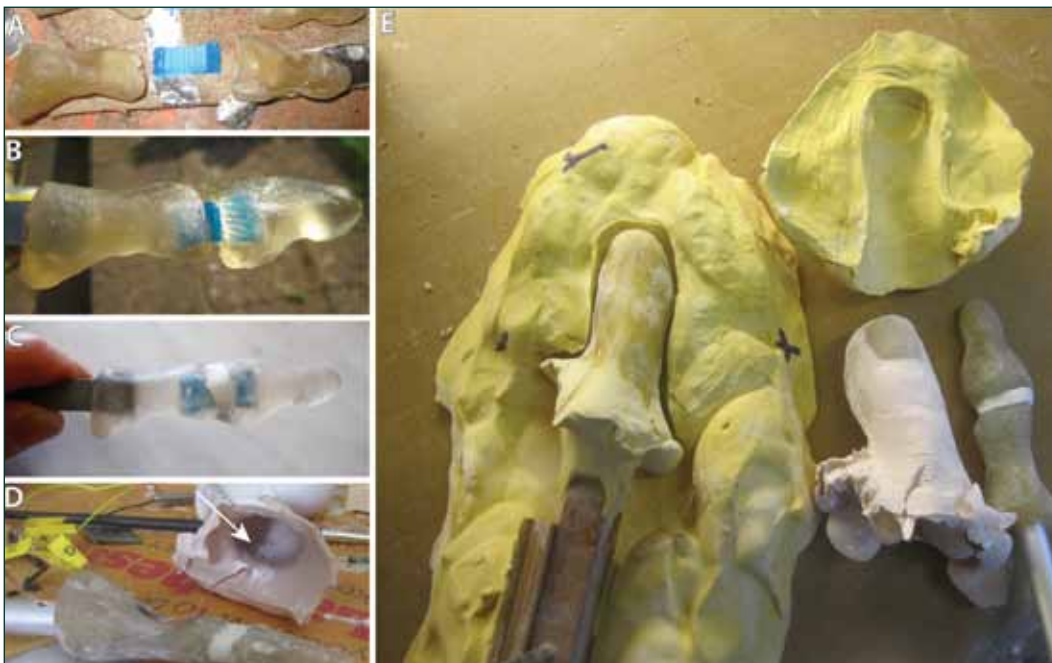
Figure 1. The authors developed a toe manikin capable of reporting the waveform and intensity of vibration imparted to its surface.
