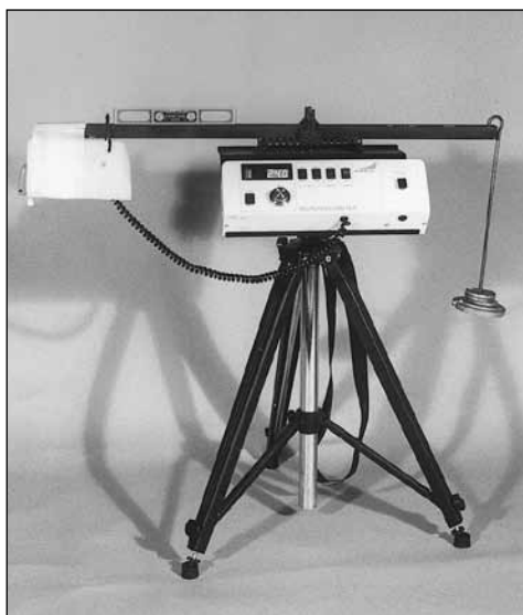
Figure 1. The rig used in the experiment comprising a Neurothesiometer, a photographic tripod stand and a beam to suspend the Neurothesiometer head.
