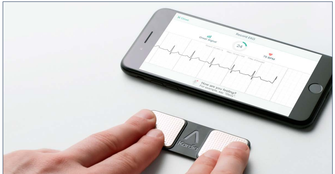
Figure 2. The AliveCor Kardia, a portable one-lead electrocardiogram device that can be used in clinic to check for atrial fibrillation.
