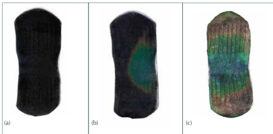
Figure 3: A Hot Spot sock a) before temperature change, b) with localised temperature change from the pressure of a hand, and c) completely colored due to heat from a hair dryer.
